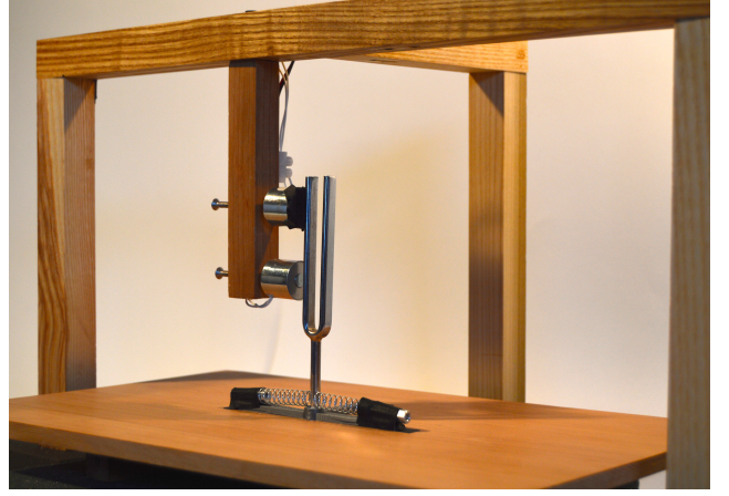
Figure 4: AAM Prototype: This implementation consists of a harmonic oscillator and acoustic amplitude modulation with parametric control of sideband components.
